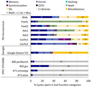
Figure 4: Breakdown of cycles spent in leaf functions.
