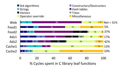
Figure 9: Breakdown of CPU cycles spent in C libraries: ML services perform several vector operations while dealing with large feature vectors.
