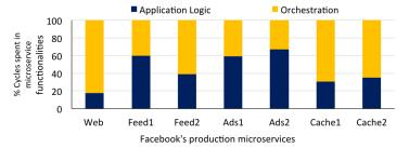
Figure 1: Breakdown of cycles spent in application logic vs. orchestration work.
