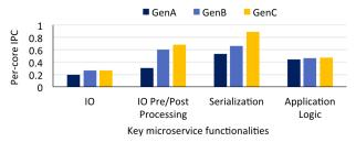
Figure 12: Cache1's IPC scaling across three CPU generations.
