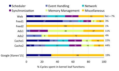
Figure 7: Breakdown of cycles spent in various kernel leaf functions: kernel scheduler, event handling, and network overheads can be high.
